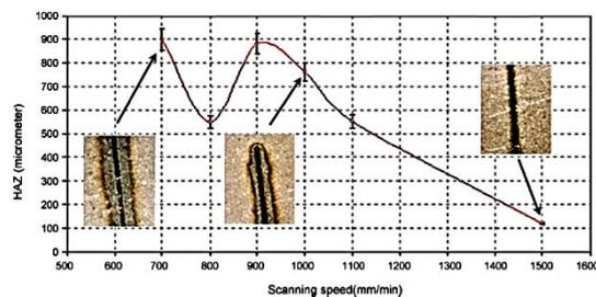
**Figure 14.** HAZ vs Speed [20]
