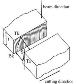
**Figure 7.** Schematic of kerf geometry.
