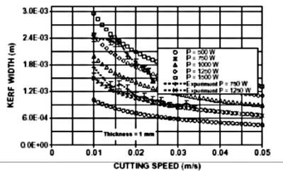
**Figure 8.** Variation of the kerf width with cutting speed [17]
