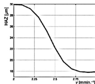
**Figure 11.** Effect of the cutting speed on the width of HAZ [18].
