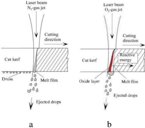
**Figure 2** Sketch of the cutting front (side view) in (a) inert gas laser cutting and (b) oxygen gas laser cutting. (Kaplan (2009))
