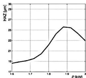
**Figure 10.** Effect of the laser power on the width of HAZ [18]
