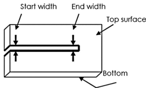
**Figure 6.** Kerf width measurements [14]
