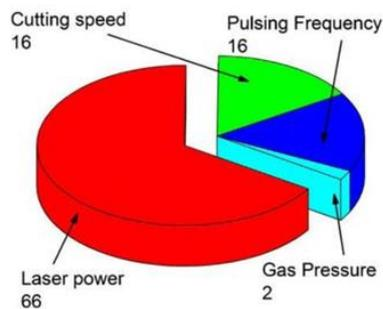
**Figure 3.** Effect of each parameter on surface roughness [8]
