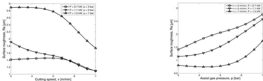
**Figure 4.** Surface roughness vs Cutting speed [10] **Figure 5.** Surface roughness vs Assist gas pressure [10]
