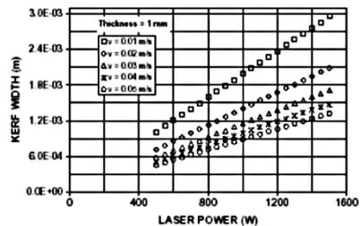
**Figure 9.** Variation of the kerf width with laser output power [17]
