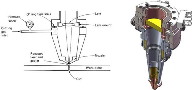
**Figure 1.** Classical gas assisted laser cutting
