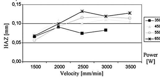
**Figure 12.** Dimension of HAZ (mm) of PMMA in function of cutting velocity for several power laser [19]
