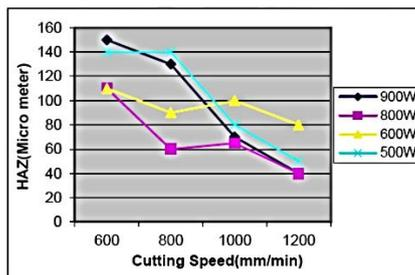
**Figure 13** HAZ Vs Cutting speed [15]
