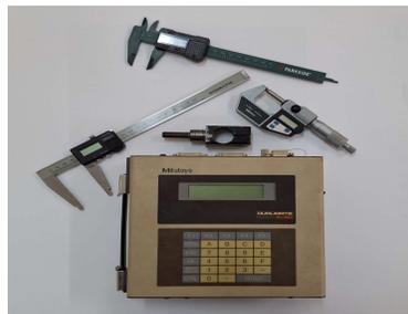
Figure 1. Universal tools for measuring dimensions.[3]
