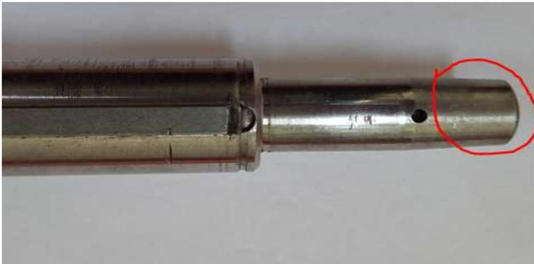
**Figure 4.** Sample of a part with an inclination on the cylindrical surface.
