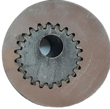
Figure 4. Prototype of a variable-eccentricity cam mechanism
