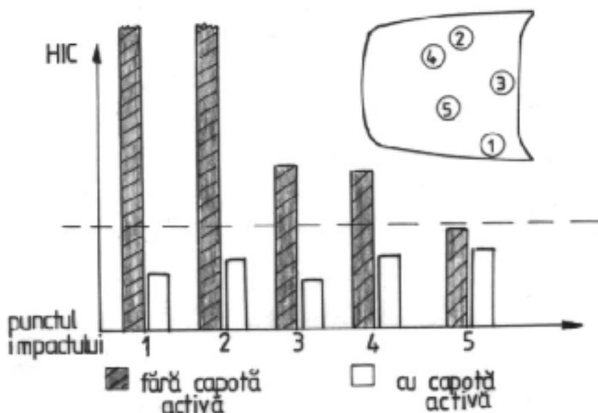
Figure 6. EuroNCAP test to test the active hood at impact with the pedestrian's head
