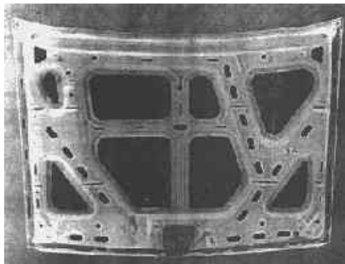
*Figure 4. Hood with rigid reinforcing structure*
