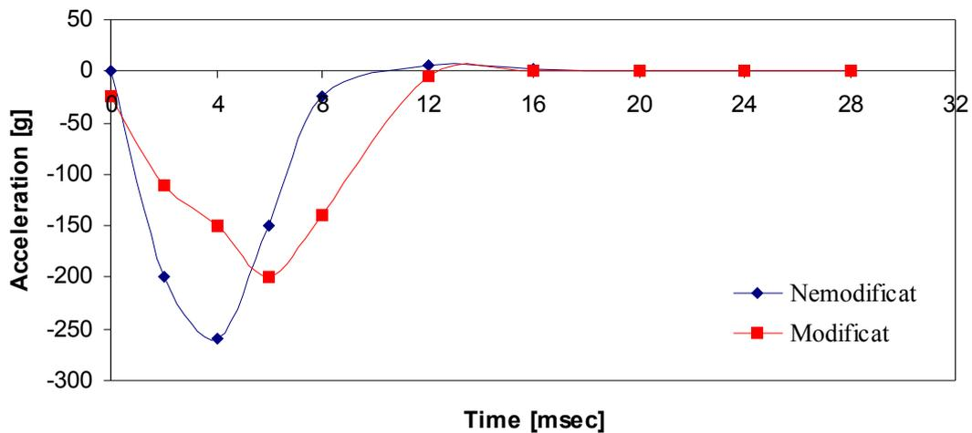
Figure 1. Effect of hood-fender area modification upon the acceleration value at impact
