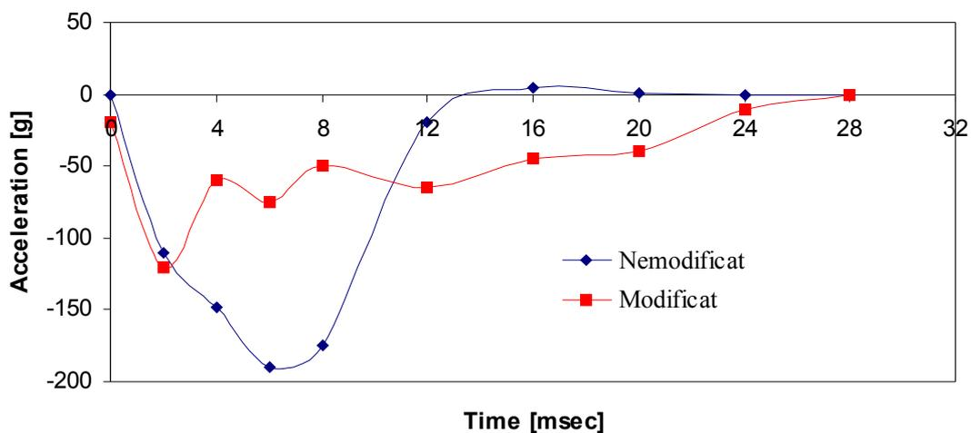
Figure 2. Effect of hood modification upon acceleration at impact
