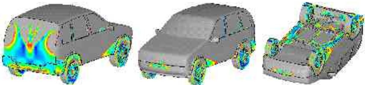
Fig. 7 - Wall shear stress distribution \tau_W , v = 60 \text{ km/h}
