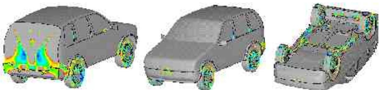
Fig. 9 - Wall shear stress distribution \tau_W , v = 120 \text{ km/h}
