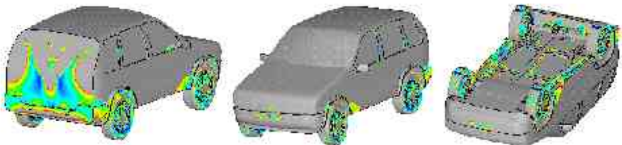
Fig. 9 - Wall shear stress distribution \tau_W , v = 120 \text{ km/h}
