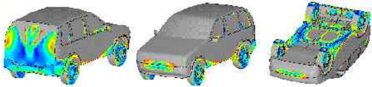
Fig. 7 - Wall shear stress distribution \tau_W , v = 60 \text{ km/h}
