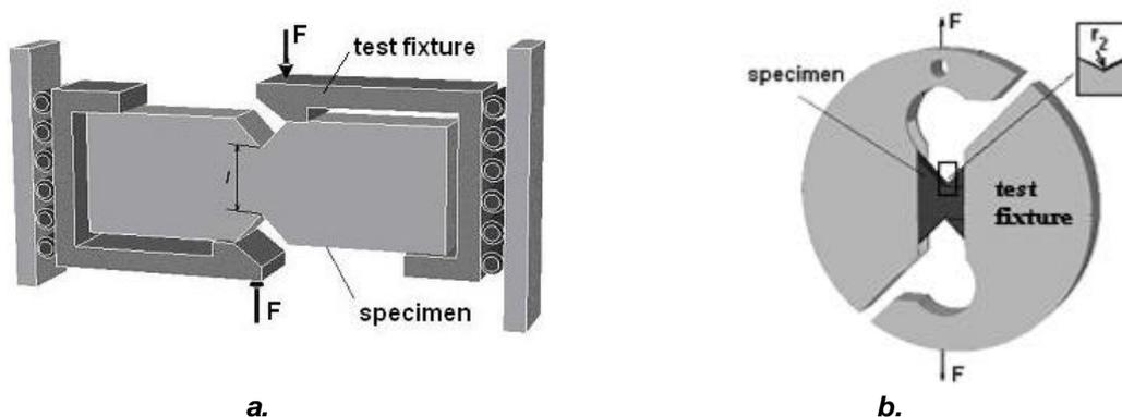
**Fig. 2. Pure shear testing devices: a. Iosipescu test method, b. Arcan test method**
