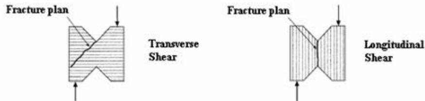
Fig. 4. Shear planes for transverse and longitudinal shear of a cortical bone
