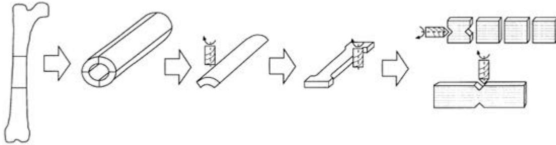
Fig. 3. Specimen preparation protocol for pure shear tests
