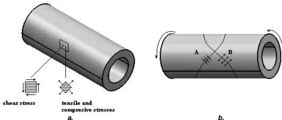
Fig. 1. Torsional loading produces: a. shear stress along and transverse to the long axis of the bone, b. compressive stress (A) and tensile stress (B)
