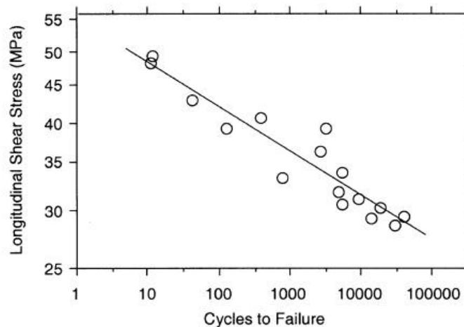
Fig. 5.  $s - N$  curve for fatigue of cortical bone in shear, [18]
