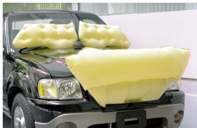
Fig. 11. Windshield Airbag proposal. Includes A-Pillar airbags (left) and actual implementation (right)
