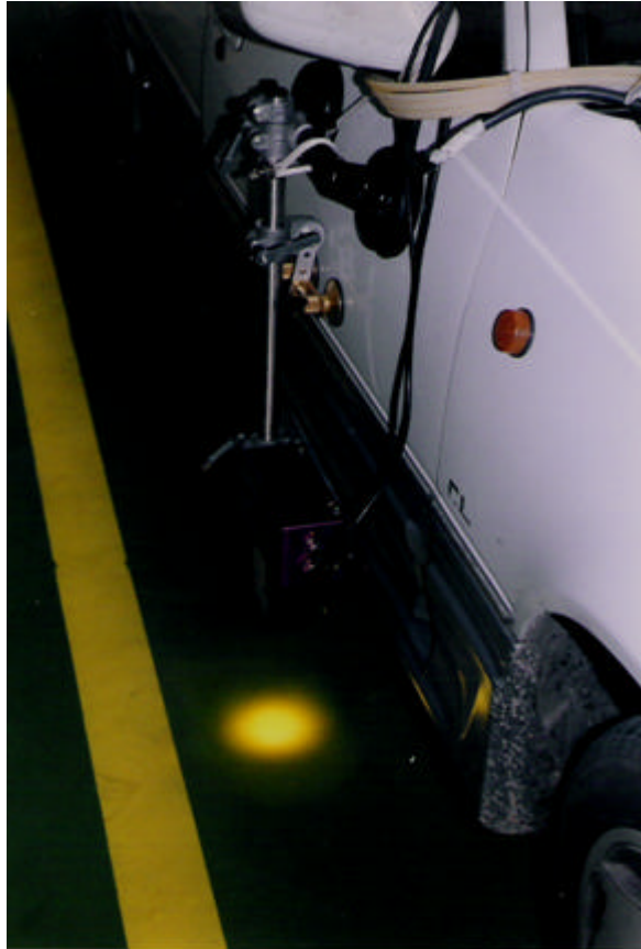
Fig.2. Speed and mileage scientific apparatus with no mechanical touching to the ground
