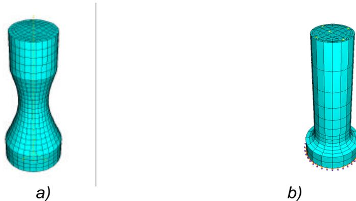
*Fig.3 FE meshes for smooth specimen (a) and notched specimen (b)*
