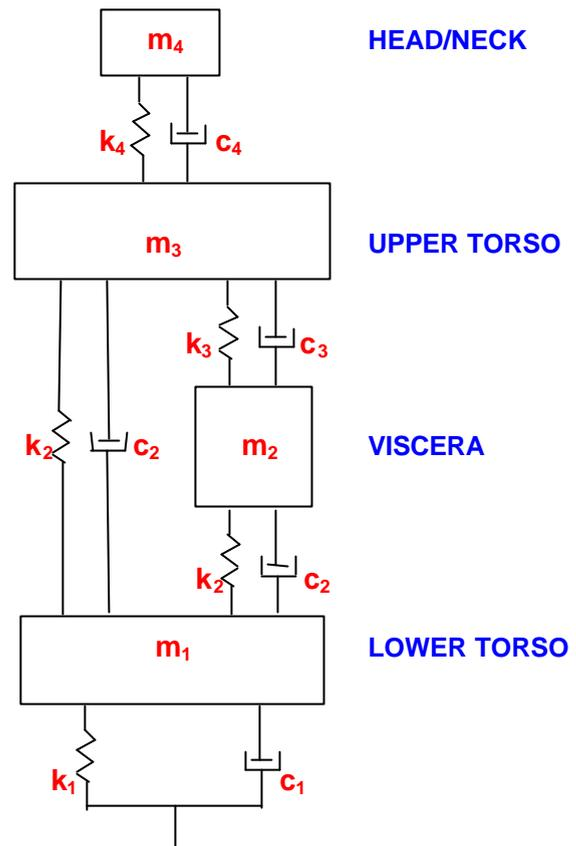
Figure 4. Vertical Low-amplitude Wan and Schimmels Linear Model
