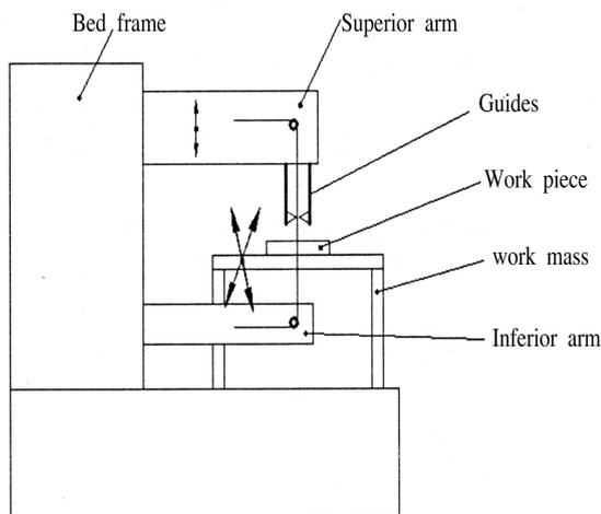
**Figure 2.** Basic structure of WCEDM system.
