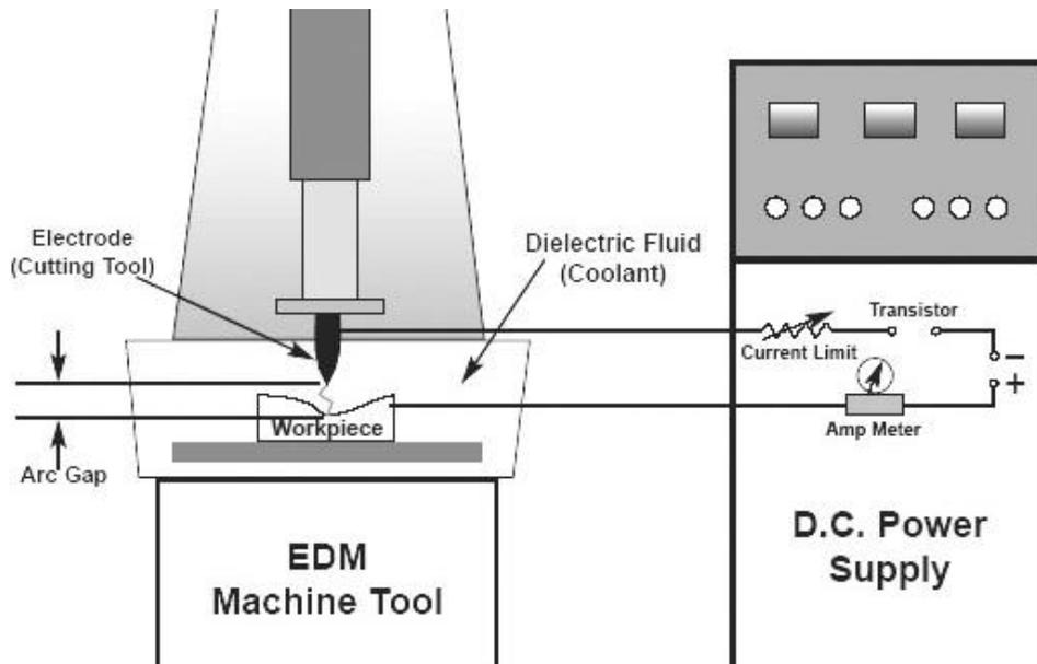
Figure 1. - Functional scheme of an Electrical Discharge Machining.
