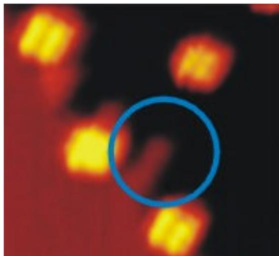
Figure 2. Image showing a nanoscopic feature molded into a monoatomically high step-edge on a copper surface.
