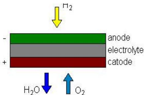
Figure 1. - Schematic of one type of fuel cell.
