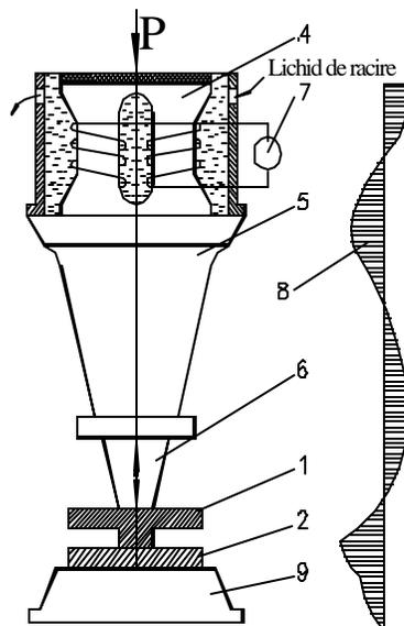
Fig.1 Ultrasonic welding scheme
