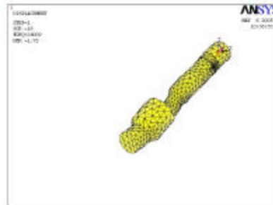
Fig. 5 Tool vibration mode at frequency  $f = 24009$  Hz.
