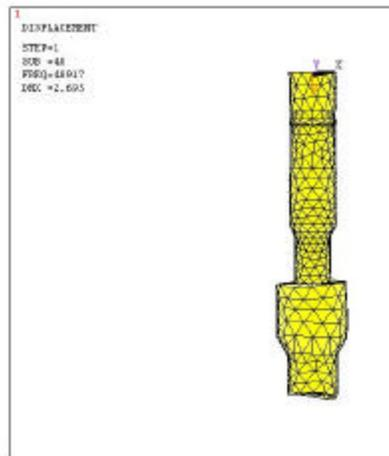
*Fig. 10 Tool vibration mode at frequency  $f = 48917$  Hz.*
