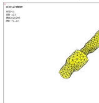
**Fig. 9 Tool vibration mode at frequency  $f = 26296$  Hz.**
