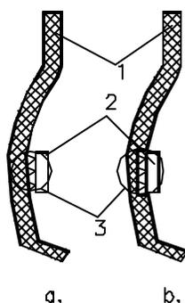
**Fig.3 Schematic of sensor welding on the rear lamp back face plastic**
