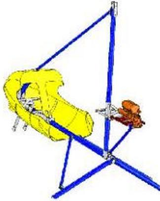
Fig. 2. The 3D model of the powered-hang-glider
