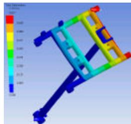
**Fig. 6. The displacement distribution over the engine's frame**
