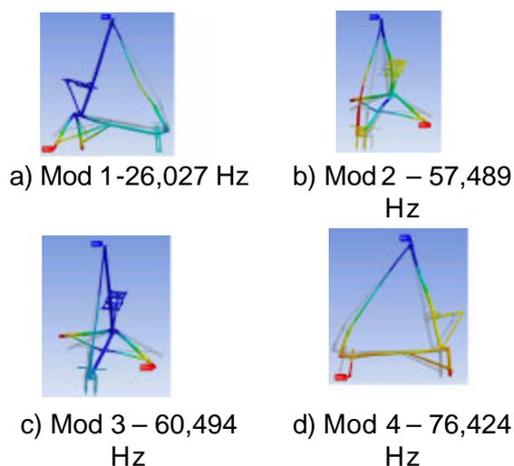
**Fig. 9. The first four vibration modes**
