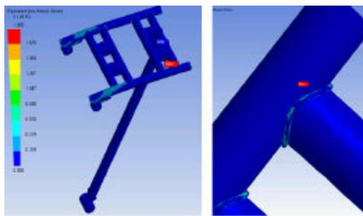
*Fig. 7. The equivalent stress distribution over the engine's frame*
