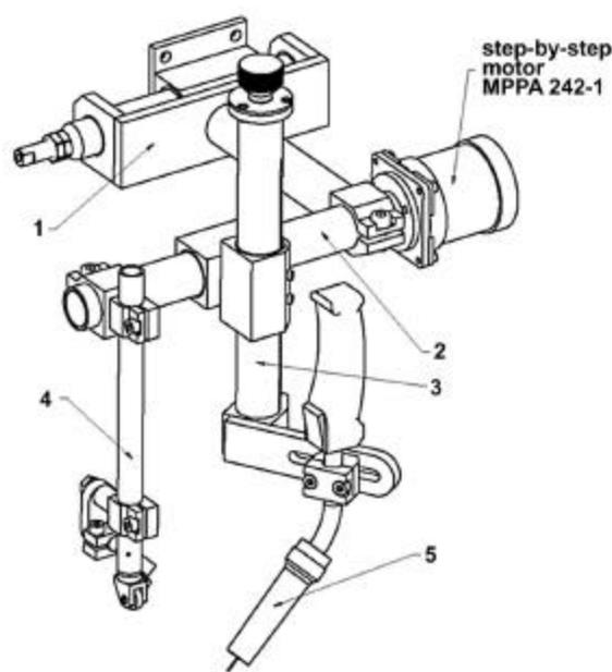
Figure 3. Positioning device for the welding head
