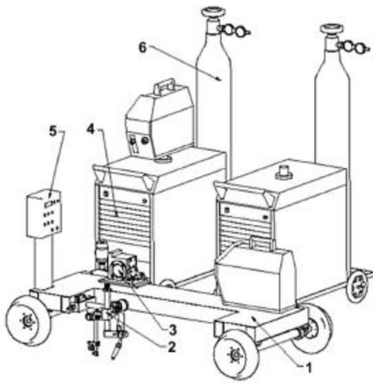
Figure 1. Mechanised installation for rails reconditioning
