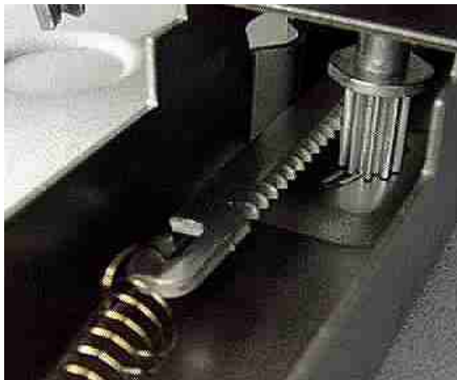
Figure 8. Rack and pinion gears from a household scale
