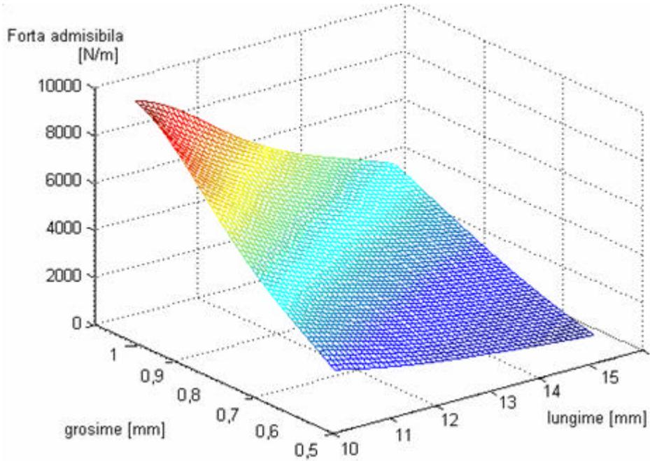
Fig.17. Diagram of the maximum admissible force versus length and thickness of the electrolytic copper electrode.
