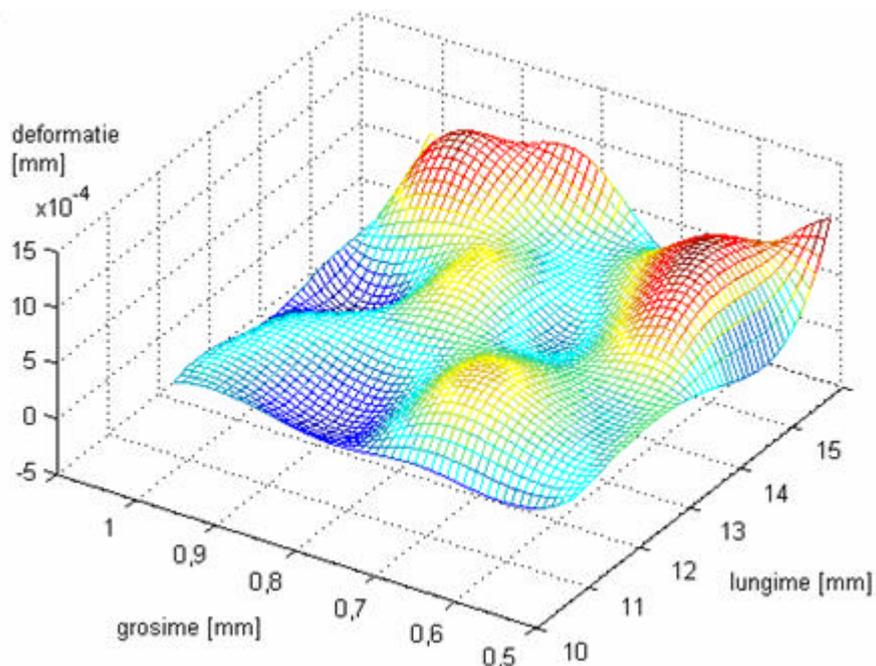
Fig.18. Diagram of the deformation versus length and thickness of the graphite electrode.
