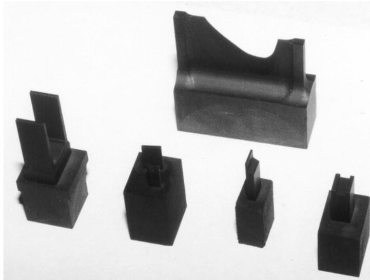
Fig.19. Graphite electrodes with thickness less than 1 mm.
