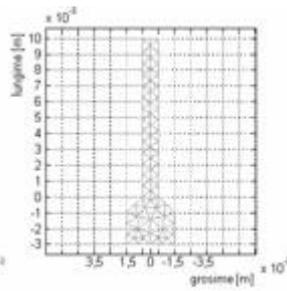
Fig.3. Finite elements digitization.
