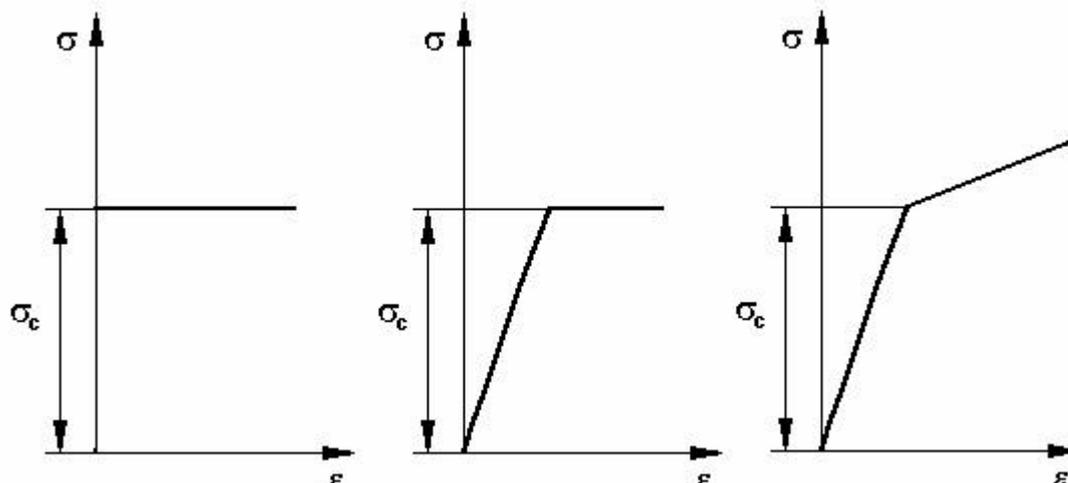
**Fig.1. The schematized flow curves: a) perfect plastic material; b) perfect plastic material with an elastic deformation; c) material with linear elastic and plastic behaviors.**
