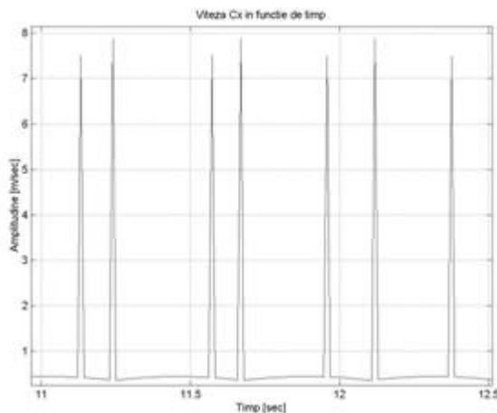
**Fig.11. The movement speed diagram of the median point (C) on the upper branch of the sorting strip, depending on time, on the Ox direction for a 1,5 seconds period.**
