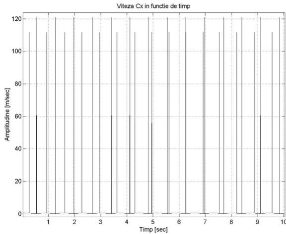
**Fig.6. The movement's speed diagram of the median point (C) on the upper branch of the sorting strip, depending on time, on the Ox direction for a 10 seconds period.**
