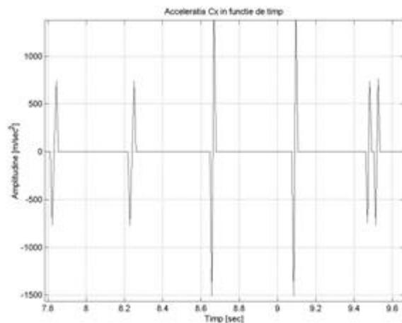
**Fig.12. The acceleration diagram of the median point (C) on the upper branch of the sorting strip, depending on time, for a 2 seconds period.**
