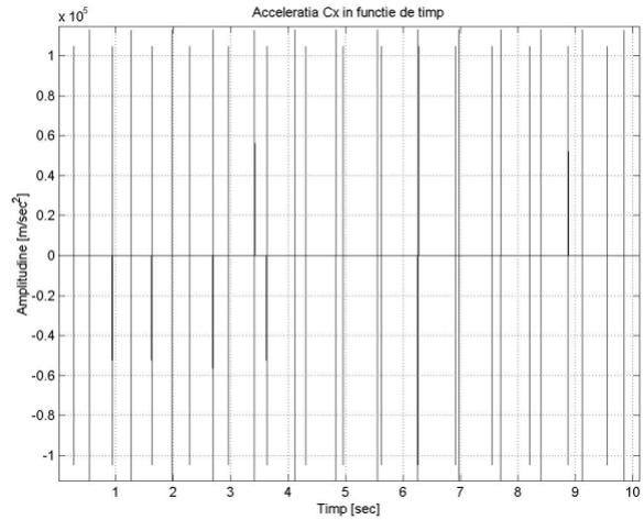
**Fig.7. The acceleration dyagram of the median point (C) on the upper branch of the sorting strip, depending on time, on the Ox direction, for a 30 seconds period.**
