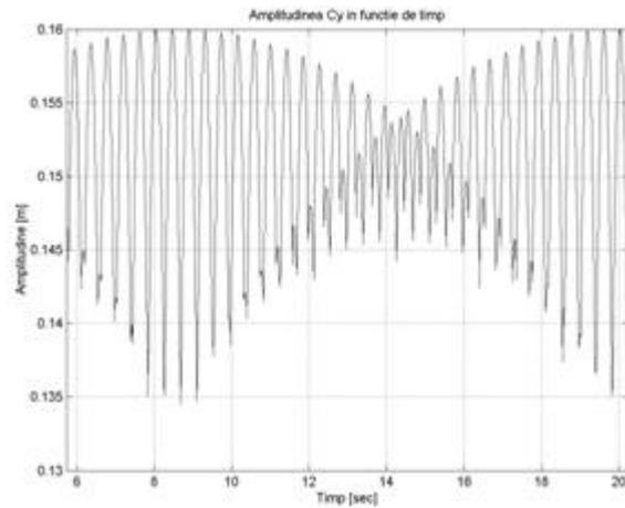
**Fig.10. The movements diagram of the median point (C) on the upper branch of the sorting strip, depending on time, on the Oy direction, for a 14 seconds.**
