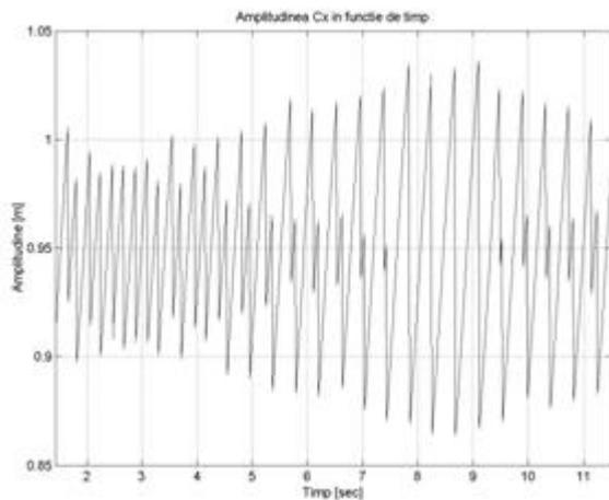
**Fig.9. The movement diagram of the median point (Cx) on the upper branch of the sorting strip, on the Ox direction, for a 10 seconds period.**
