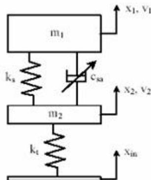
**Figure 3. Semi-Active Equivalent Model**
