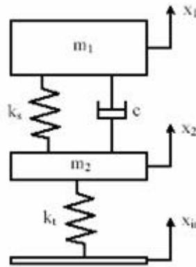
Figure 1. Passive suspension
