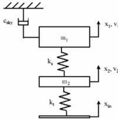
**Figure 2. Skyhook Damper Configuration**
