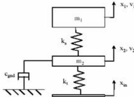
**Figure 4. Groundhook Damper Configuration**
