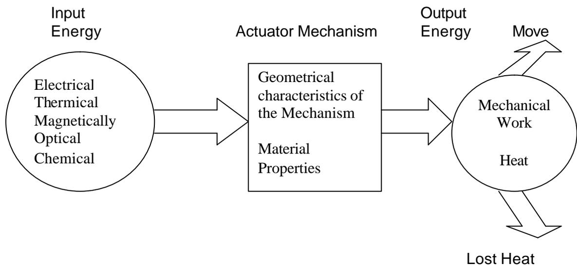
Fig.3. The diagram of an Actuator structure
