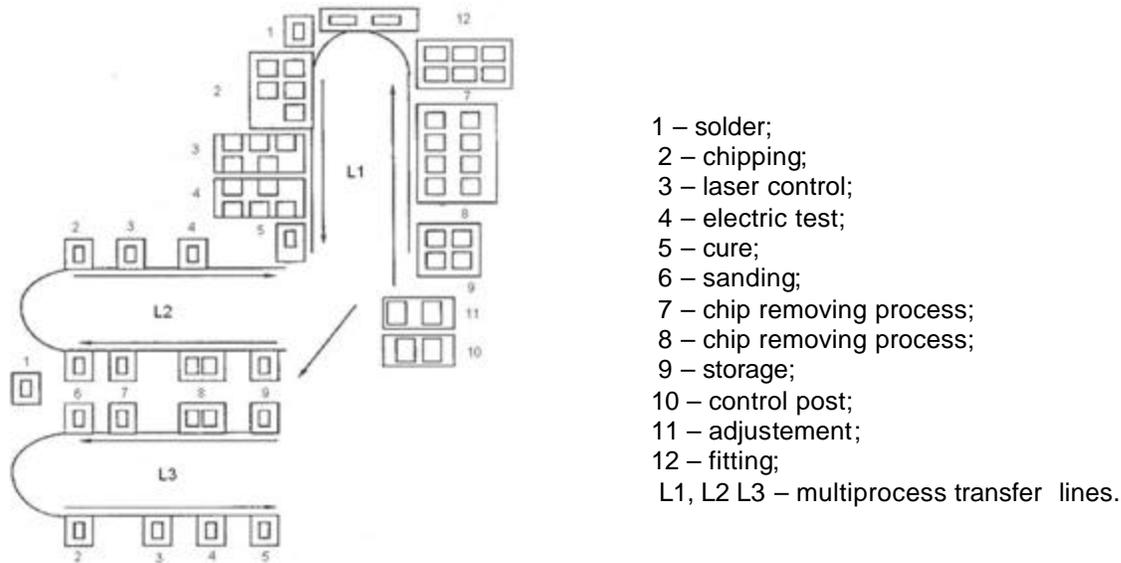
**Fig. 1. Example of multiprocess cell structure**
