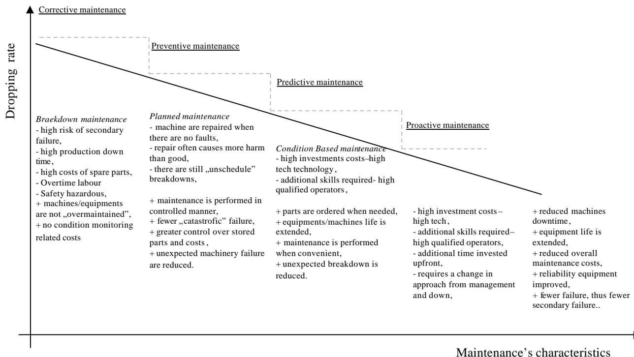
Fig. 2. Maintenance methods, characteristics
