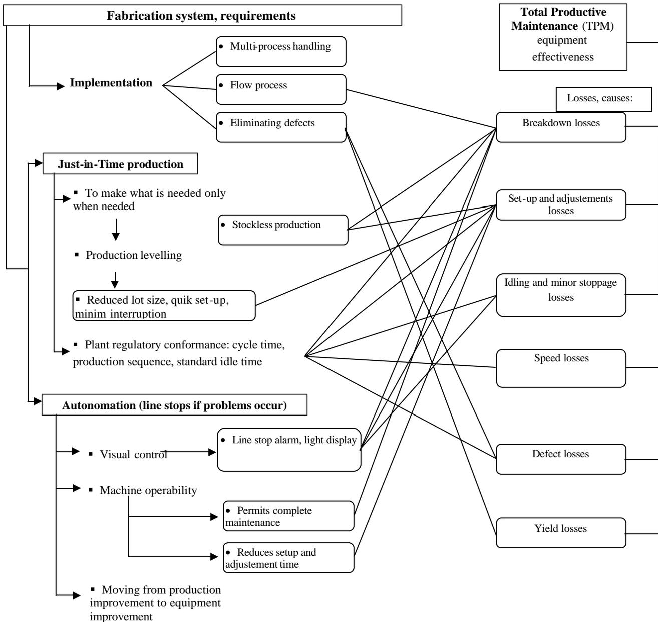
Fig. 3. TPM machines/equipments requirements and losses causes
