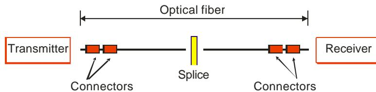
Fig. 1. Optical communication system
