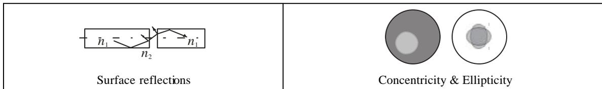
The difference between the axis of the core and the axis of the cladding is expressed as the “concentricity” of the fiber. This means that unless one does something to align the cores simultaneously with making the connection, there will be a (random) misalignment, and hence a loss, imposed by the concentricity error [3]. The major improvements in optical transmission was due generally to better fiber manufacturing as much as to better connectors and connection techniques .
