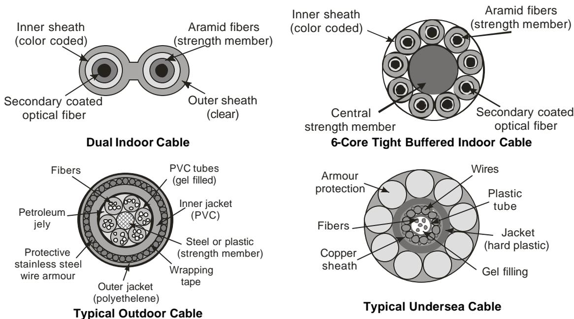
Fig. 2. Typical fiber optic cables [3]
