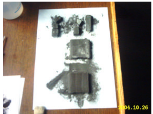
Fig.12. The prisms obtained with SLS method
