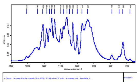
Fig.8. The position of bands for HA with heat treatment 3h at  $900^\circ\text{C}$
