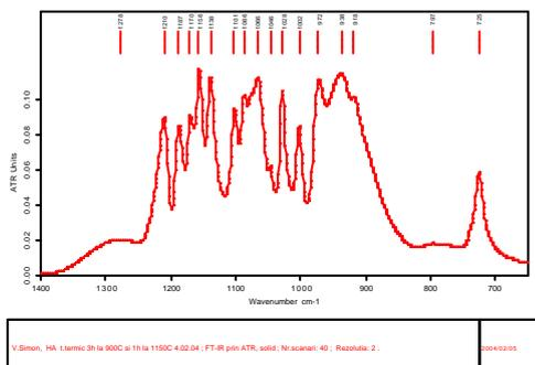
Fig.7. The position of bands for HA with heat treatment 3h at  $900^\circ\text{C}$  and 1 h at  $1500^\circ\text{C}$
