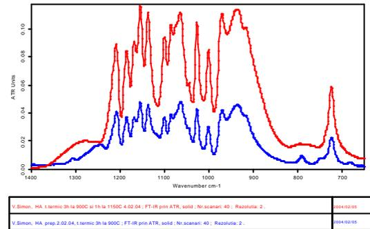
Fig.6. FT-IR spectrum by reflexion registers in domain  $600\text{-}1400\text{ cm}^{-1}$  for HA
