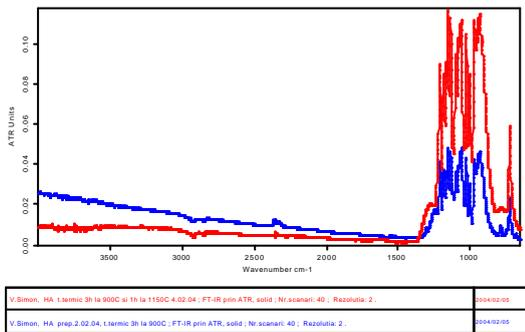
Fig.5. FT-IR spectrum by reflexion registers in domain  $600\text{-}4000\text{ cm}^{-1}$
