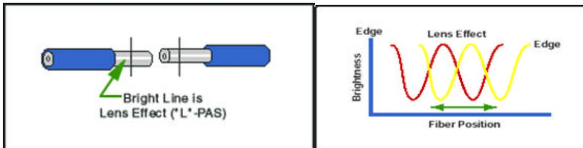
Figure 5 -Lens - Profile Alignment System (L-PAS) Video Program
