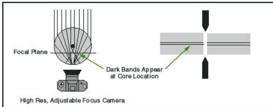
Figure 4 The PAS System "sees" the core by detecting the refraction of light caused at the core-cladding.
