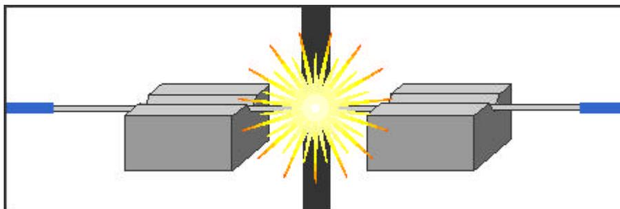
*Figure 1 - Fusion Splicing*
