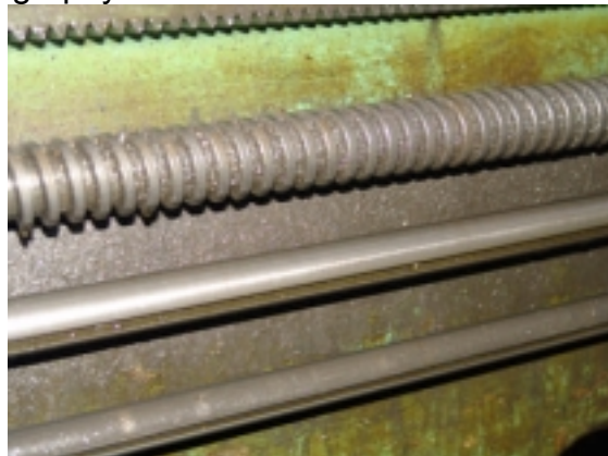
Fig. 3 Tie bar with grooved wedge of a normal lathe
