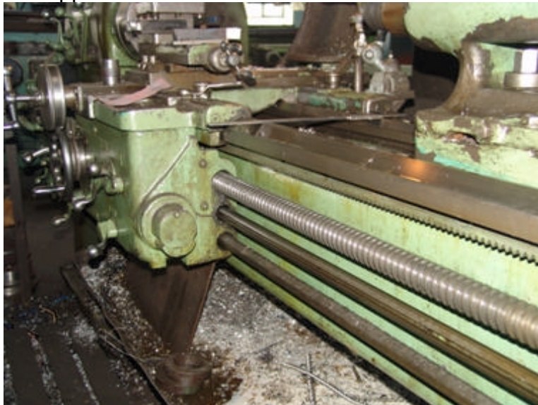
Fig. 5 Opposed on-off mechanism with hexagonal tie bar at a Iosif Ranghet lathe
