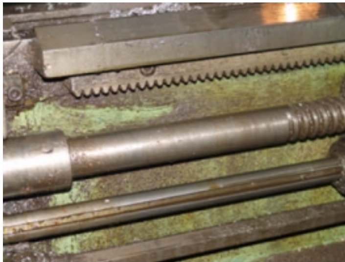
Fig. 1 The Iosif Rangheț lathe with the adjustment of the on-off mechanism of the main shaft
