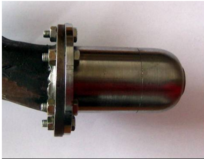
Figure2. The new injector for Pelton turbine
