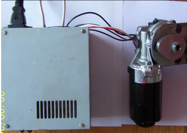
Figure4. D.C. motor and power supply for cam mechanism
