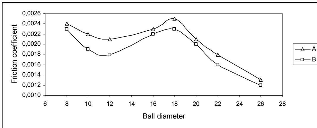
Fig. 2. The rolling-friction coefficient for different ball sizes (sample A and B)
