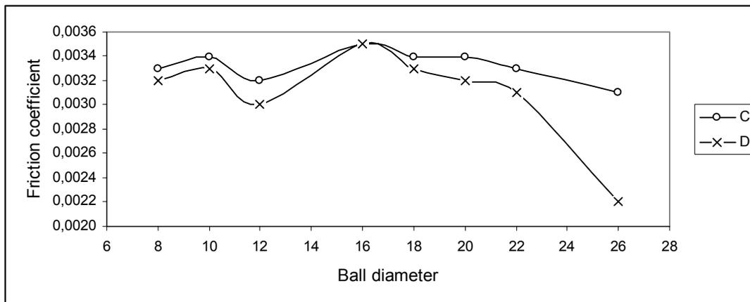
Fig. 3. The rolling-friction coefficient for different ball sizes (sample C and D)
