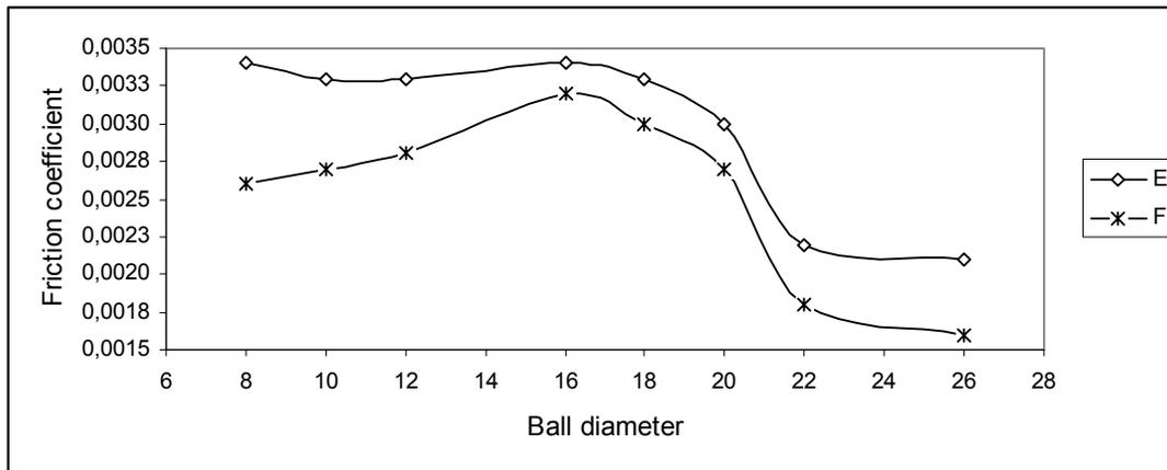
**Fig. 4. The rolling-friction coefficient for different ball sizes (sample E and F)**
