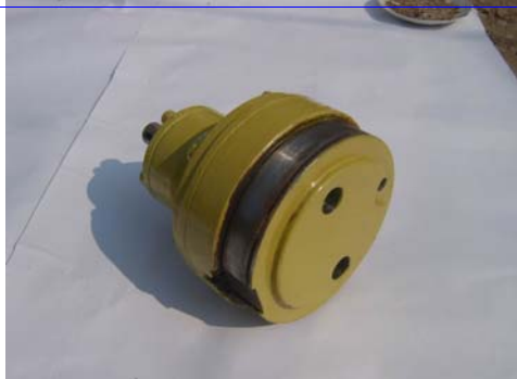
Fig.5 Hydraulic motor or hydraulic pump elliptic piston
