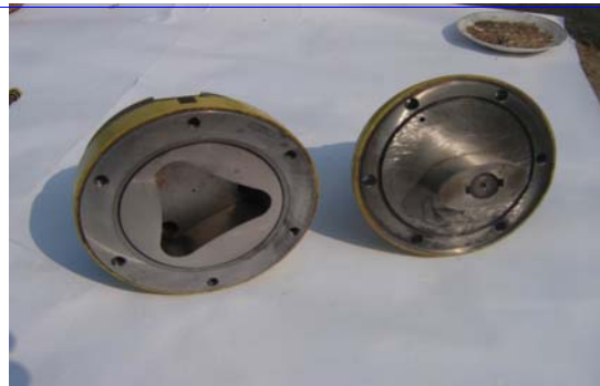
Fig.6 The volumetric chamber and rotative elliptic piston
