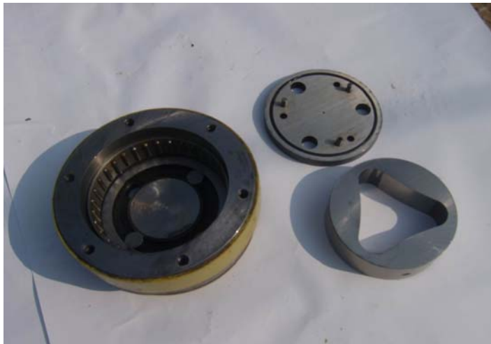
Fig.7 The distribution is made by flange clasped on the rotative volumetric chamber
