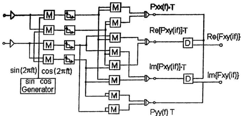
Picture 2. Logical scheme of Multiplying the Fourier transformed equations of the signals [2], [4]
