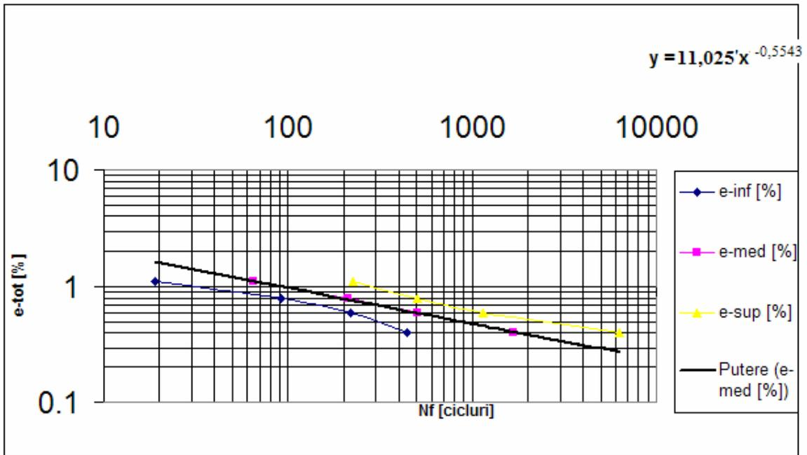
Fig.5. Manson-Coffin Equation from 16Mo5.3b steel, the thermomechanical fatigue tests are conducted in temperature range 60°↔540°C, without soaking period at maximum temperature.
