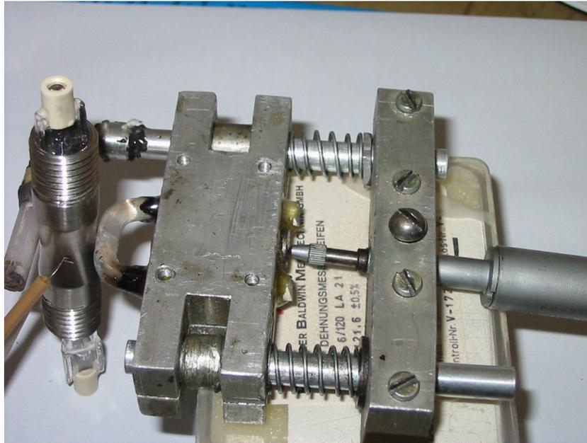
**Fig. 1. Diametrical deformation transducer in contact with the test specimen**
