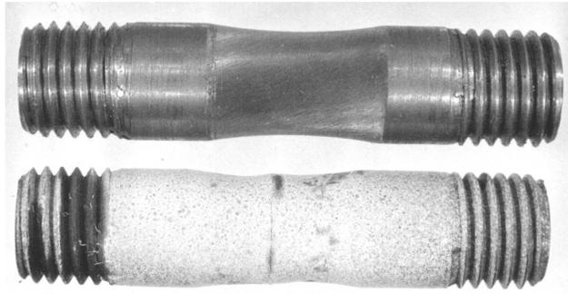
*Fig.2. The initial and final form of the thermal fatigue test specimen*
