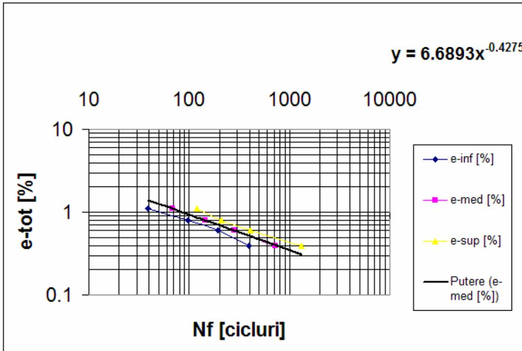
Fig.4. Manson-Coffin Equation from 16Mo5.3b steel, the thermomechanical fatigue tests are conducted in temperature range 60°↔540°C, with 600 second soaking period at maximum temperature of 540°C.
