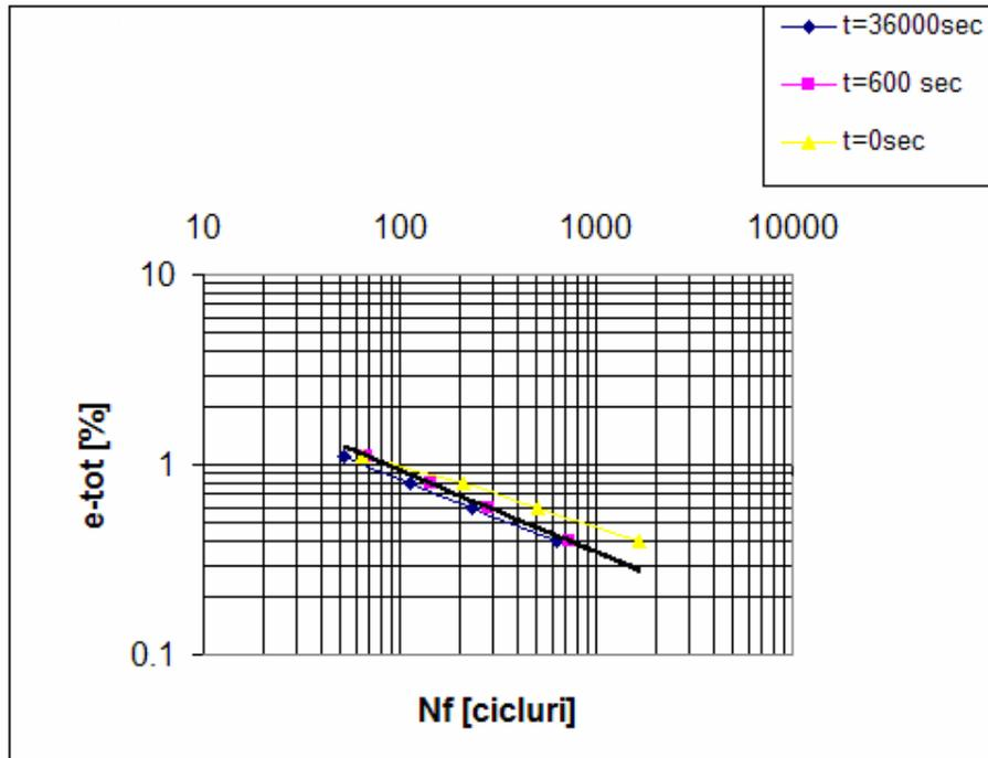
Fig.6.The comparasion for the medium line regresion, in the third previous cases of thermomechanical fatigue tests
