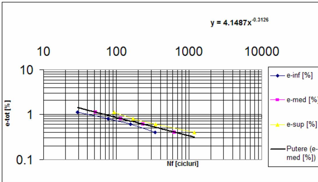
Fig.3. Manson-Coffin Equation from 16Mo5.3b steel, the thermomechanical fatigue tests are conducted in temperature range 60°↔540°C, with 3600 second soaking period at maximum temperature of 540°C.
