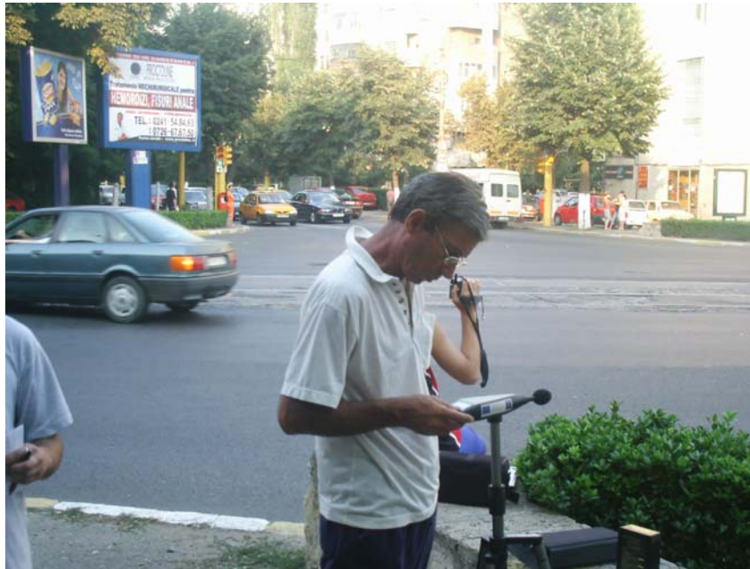
Fig. 7. Measurement of the traffic noise pollution with the 2237 Sound Level Meter
