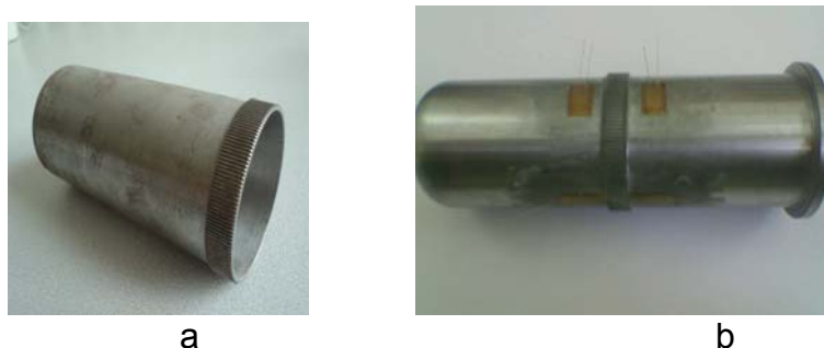
Fig. 3 Flexible gear wheel a. at classical harmonic drives; b. at hermetized harmonic drives
