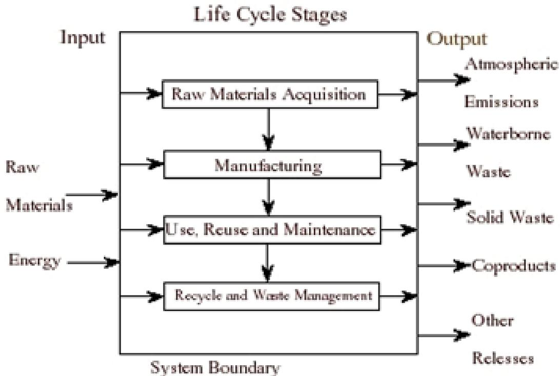
**Fig. 2 Defining system boundaries (from G.A.Keoleian, Dan Menerey and M.A. Curran, 1993, *Life cycle design guidance manual*, EPA/600/R-92/226, January, Cincinnati)**
