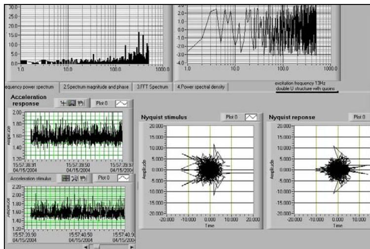
Fig. 11. Acceleration characteristics, the transfer function and Nyquist characteristics in the process of milling a 35 mm thick beech plate
