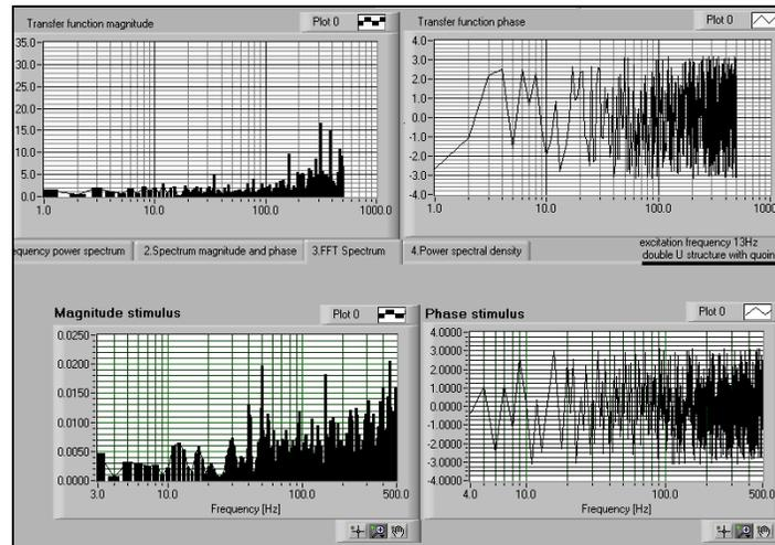
**Fig. 12. Fourier's rapid transform of the impulse and the transfer function for the operation without the cutting process**
