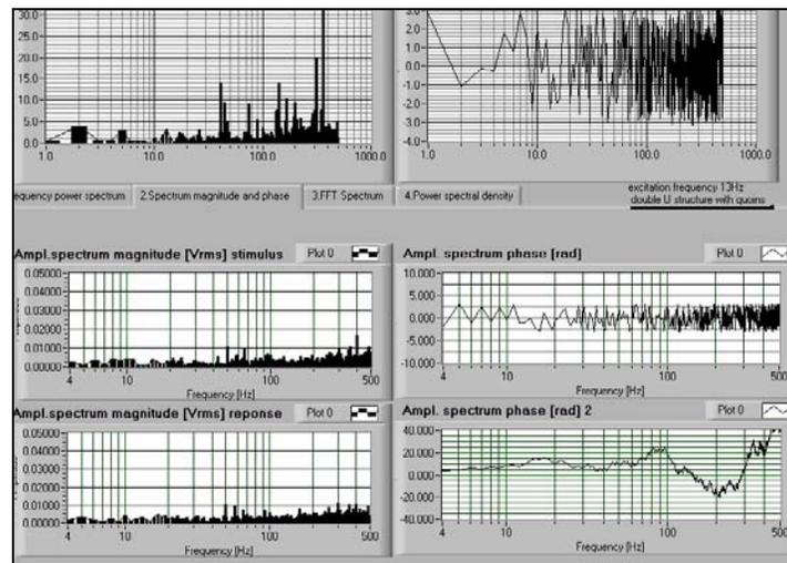
**Fig. 8. Fourier's spectrum of the electric motor and of vertical slide transfer function when the machine is in service with feeding motion and exhaustion system during the process of cutting a 40 mm thick beech plate**
