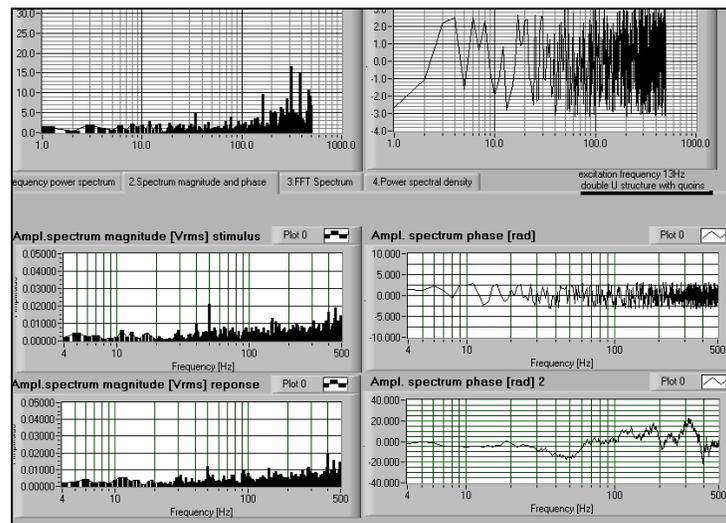
Fig. 10. Fourier's spectrum of the electric motor and vertical slide transfer function with feeding motion and exhaustion system during the process of cutting a 35 mm thick oak plate
