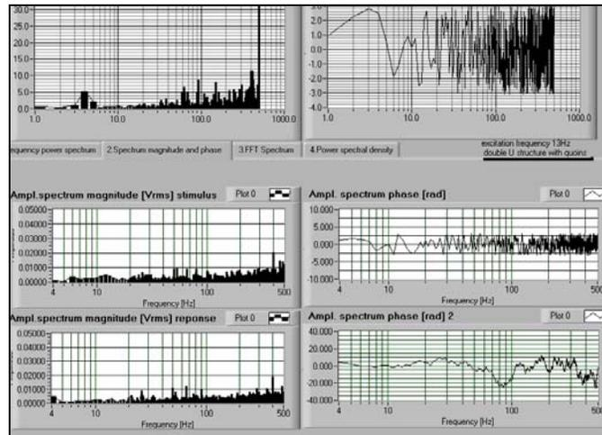
**Fig. 6. Fourier's spectrum of the electric motor and of vertical slide transfer function when the machine is in service without feeding motion and exhaustion system**
