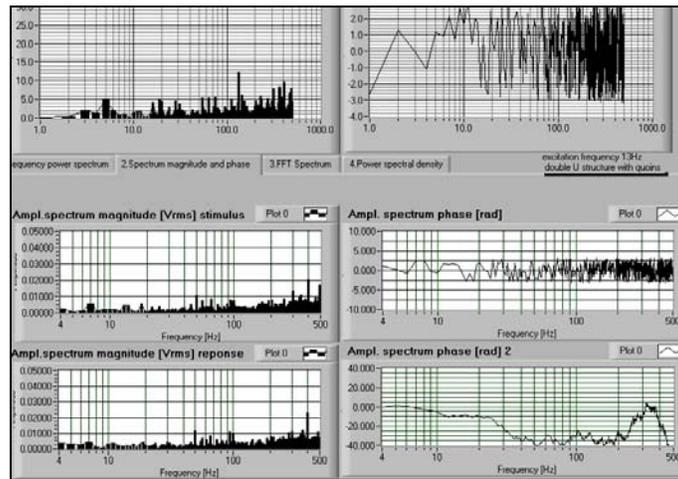
**Fig. 7. Fourier's spectrum of the electric motor and of vertical slide transfer function when the machine is in service with feeding motion and exhaustion system**
