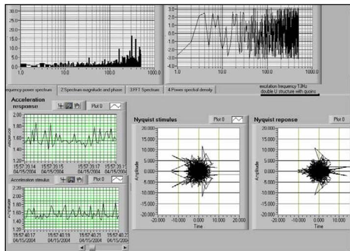
**Fig. 13. Zoom of the acceleration, transfer function and Nyquist characteristic in the process of cutting a 35 mm thick oak plate**
