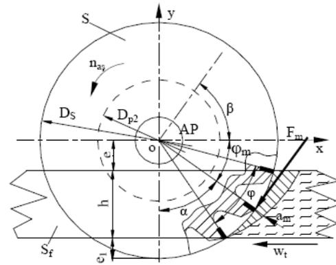
Fig. 2. Geometrical and technological parameters of the disk miller cutting
