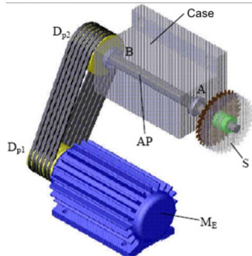
Fig. 3. The structure of the main kinematic chain
