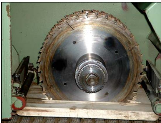
**Fig. 5. Arrangement of disk millers on the main shaft**
