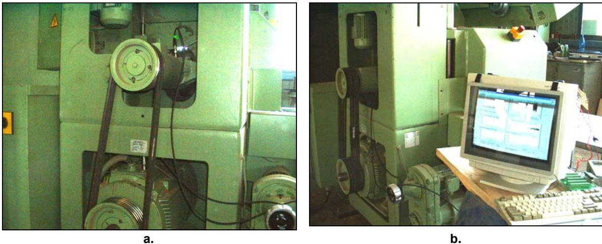
**Fig. 4. Experimental stand: a - accelerometers location; b - data acquisition system**
