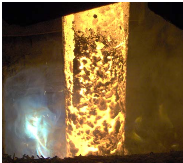
Fig.2. Mode of adding the micro-coolants in the mould of the continuous casting machine.
