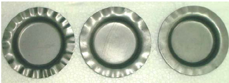
Fig.3. Variation of the wrinkles depending on the retaining force
