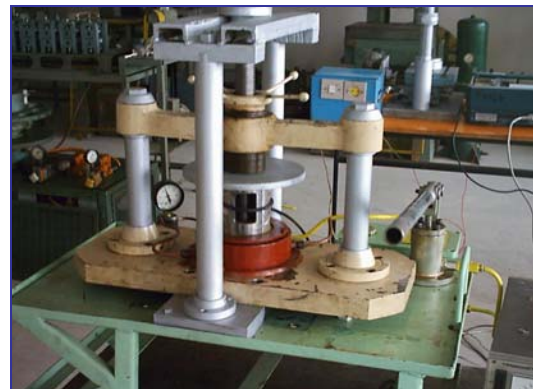
Figure 5. Device by hydroforming corrugated
