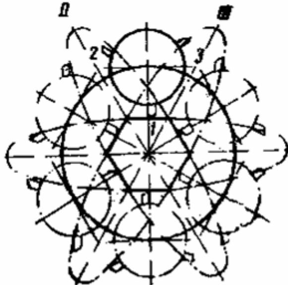
*Fig.1. Diagram of a square turning method.*
