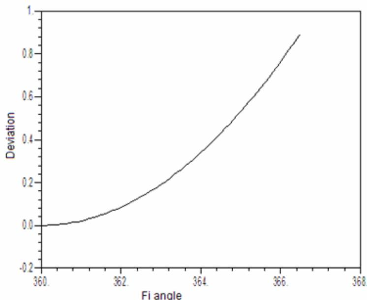
**Fig.14. The deviations on the abscissa direction for a hexangle with 14 mm size of jaw.**
