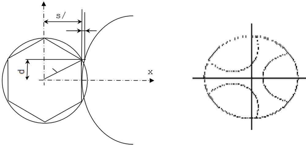
Fig.10. Basic diagram for hexagon side calculus. Fig.11. Three strands plotted on the pitch line.
