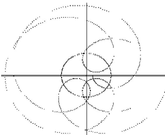
**Fig.9. Elongated epicycloids obtained from two tools on the  $90^{\circ}$  staggered – one rotation.**
