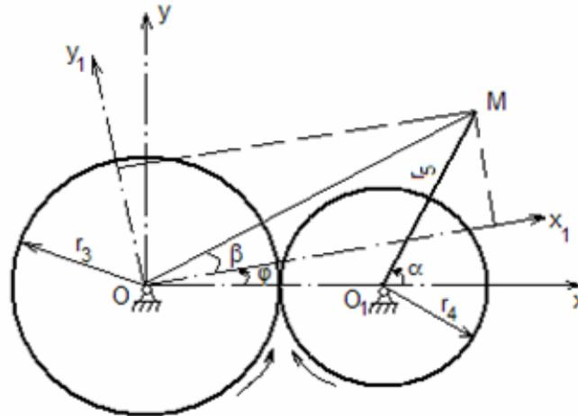
Fig.2. Basic diagram for epicycloids generation.
