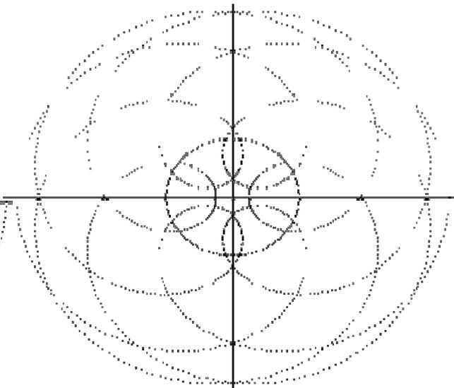
**Fig.10. Elongated epicycloids obtained from two tools on the  $90^{\circ}$  staggered – two rotations.**
