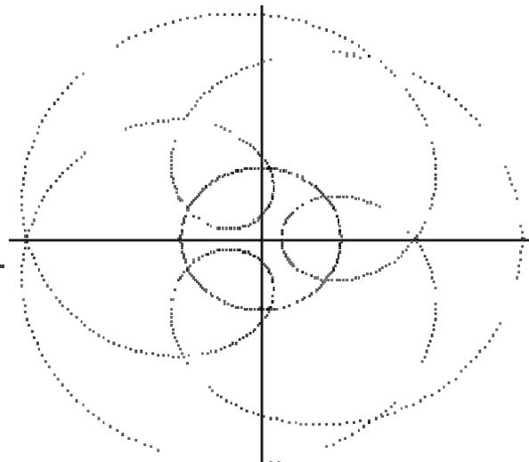
**Fig.8. Elongated epicycloids obtained from one tool – two rotations.**
