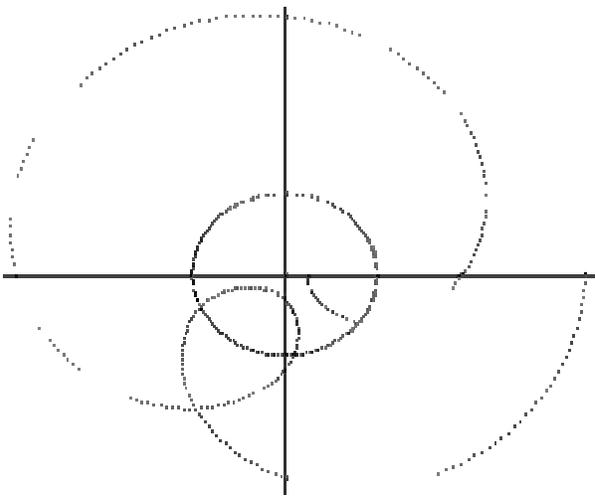
**Fig.7. Elongated epicycloids obtained from one tool – one rotation.**
