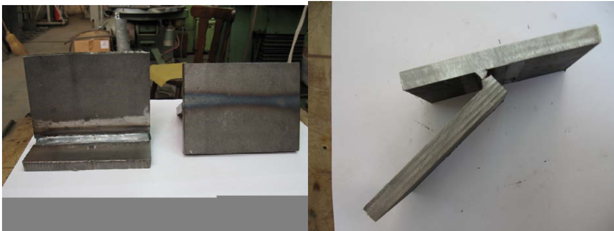
Fig.2 Sample for procedure 135, position PB; a-welded, b-broken
