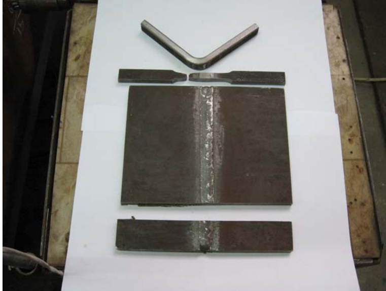
Fig.1 Sample procedure 135, position PA ; trial for pull and bend.
