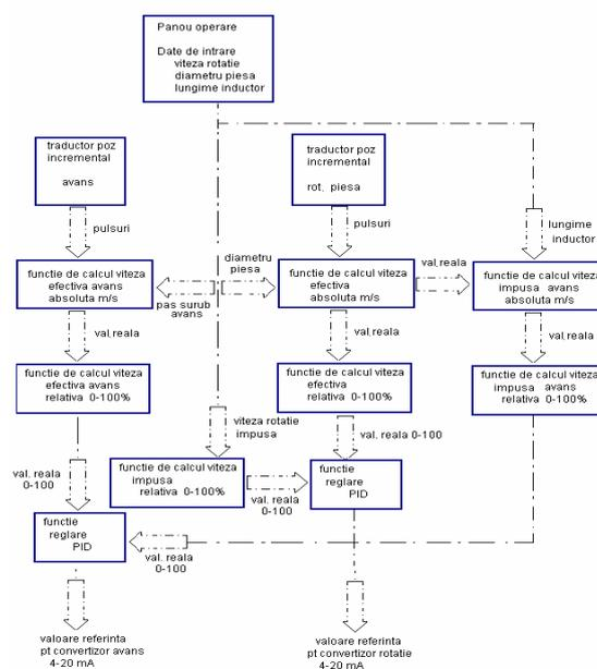
**Fig. 3. Automatic synchronism programme of the two rotation-translation successive hardening movements**
