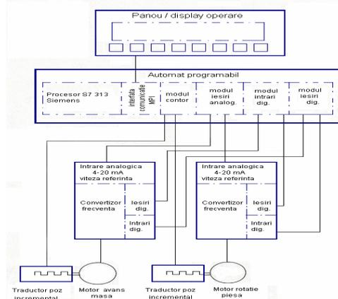
**Fig. 2. Block diagram for the automation of the IMCA type part carrying away device**
