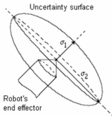
**Fig. 3 – Disc shaped uncertainty surface model**
