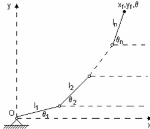
Fig. 7 – Generic serial planar robot
