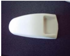
Figure 2. The prototype part model made by SLS process was used as master model for the manufacturing of the Metal Spraying mould [4]
