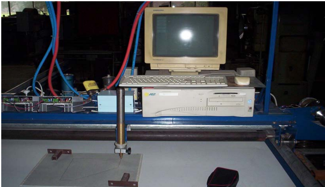
Figure 2.1. Front view of the CNC machine system for the mechanised oxygas cutting
