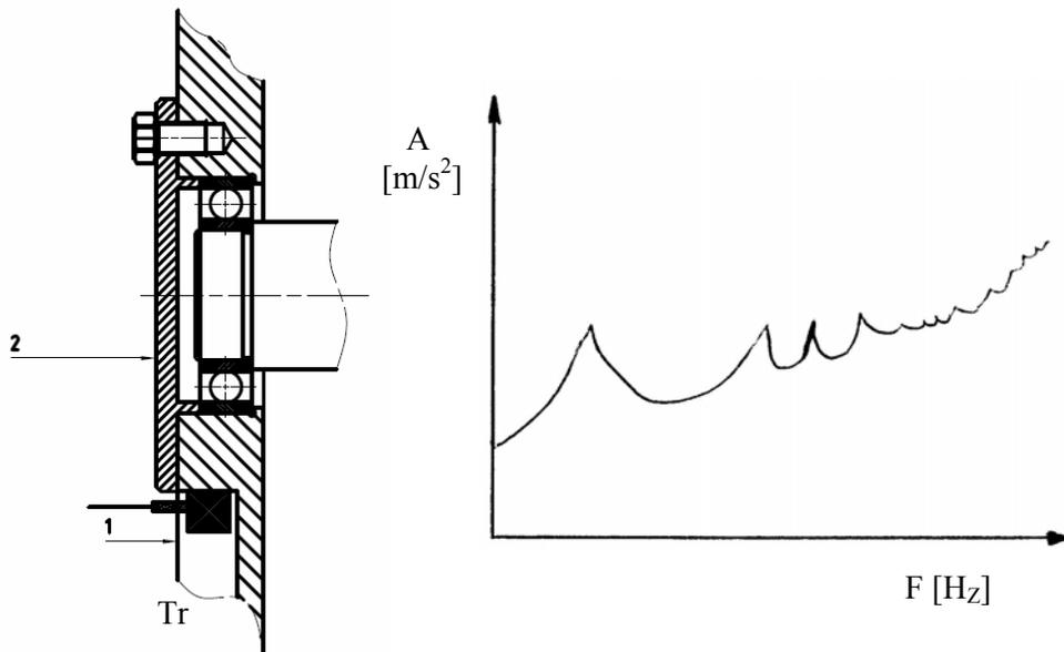
*Figure 1. Solutions for arranging the translators on the shafts' bearings; bearing structure*
