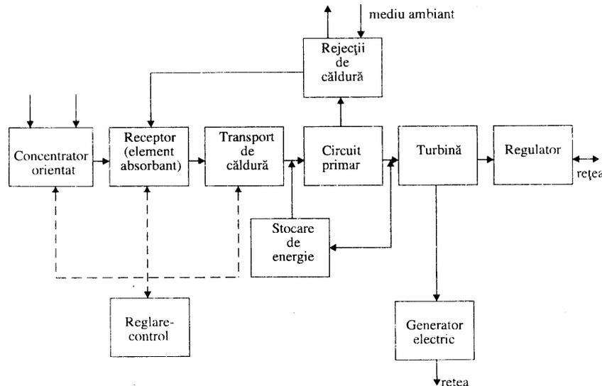
Fig.2. Main block diagram of a power plant based on helio-thermodynamic cycle.
