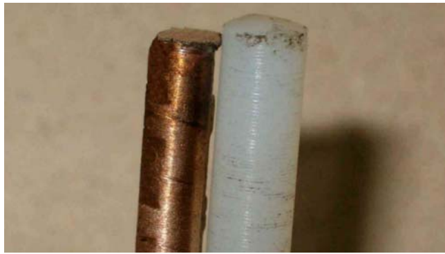
Figure 6- Comparison between bronze and Ertalon66SA test specimen
