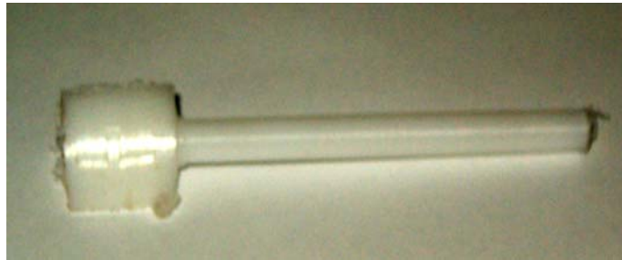
Figure 1- Test specimen for attrition behaviour
