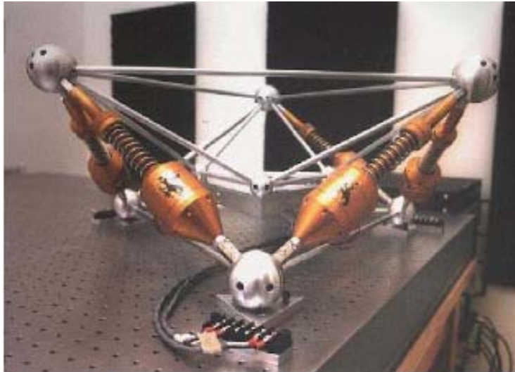
Fig. 6. University of Wyoming/JPL hexapod with internal springs
