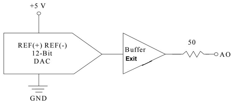
**Fig. 7. The analog output circuit**
