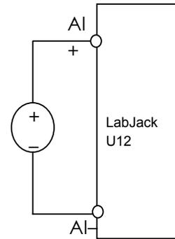
**Fig.3. The voltage signals' differential connection**
