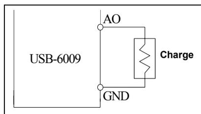
**Fig. 6. Charge connection**
