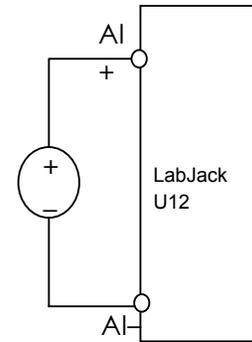
**Fig.3. The voltage signals' differential connection**
