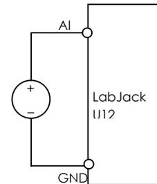
**Fig.5. Single-pole Connection**
