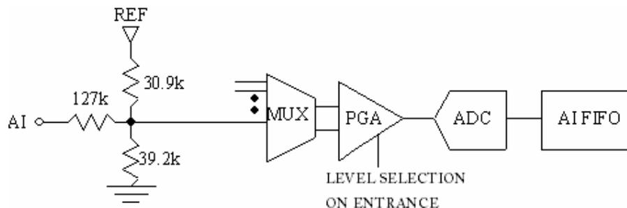
Fig.2. The analog input circuit of LabJack U12
