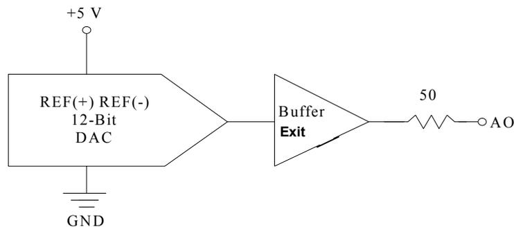
**Fig. 7. The analog output circuit**
