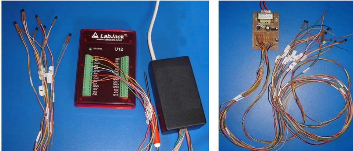
**Fig.9. Data acquisition card and the LM 35 sensors**
